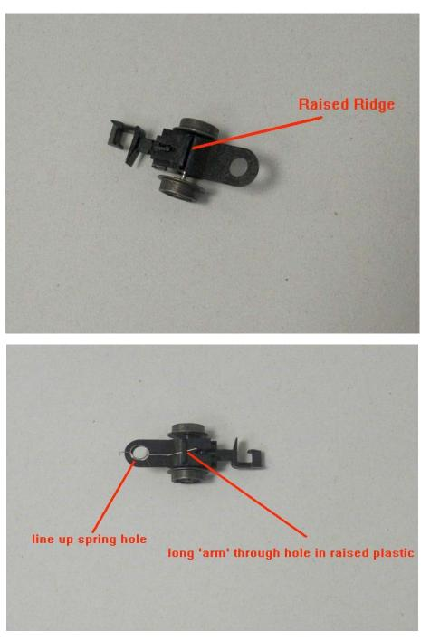
Offer up the whole unit to the bogie pivot point node on the underside of the chassis, then carefully place the new 'keeper plate' into the position of the old one locating the vertical part of the spring in the tiny hole (D) that is just behind the screw hole (C). (this helps give the spring its tension).
