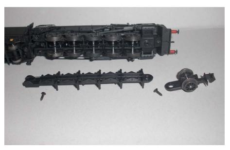
Take the tension spring, and locate the long end into the hole in the middle of the raised 'lip' on the topside of the replacement bogie frame. Line up the hole in the spring with the pivot hole in the bogie frame.
