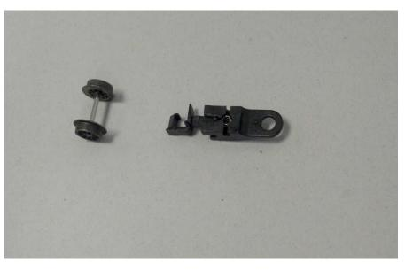
Take the replacement bogie and put the spring into the hole in the new bogie frame. (if you lose the spring, that is why there is a spare in the kit). Replace the wheel set into the new bogie frame.
