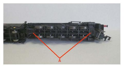
The front bogie can now be removed. Unclip the wheels from the front bogie, and also the tension spring that is in the recess under the axle.
