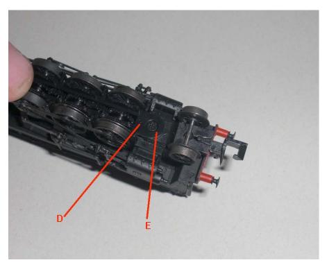
All that remains to do is carefully unclip the brakegear from the existing 'keeper plate' (you may have to cut the 2 rear rods to allow you to do this) and fit to the new 'keeper plate' , gluing back the rods into place on the new plate.
